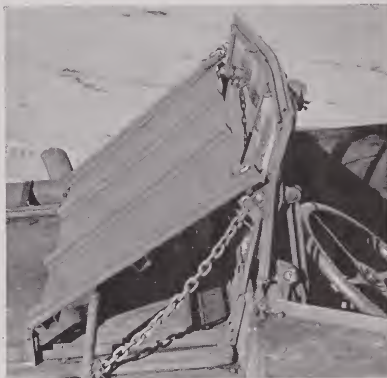
FIGURE 32. Effect of surf impact on windshield reinforced with early field modification kit.
